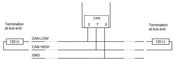
The cable specification is about 120  $\Omega$ .
