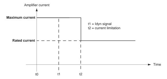
The maximum current duration before the release of the Idyn signal output (t1 - t0) and before the rated current limitation (t2 - t0) is calculated the same way as for the **Fusing** mode.
