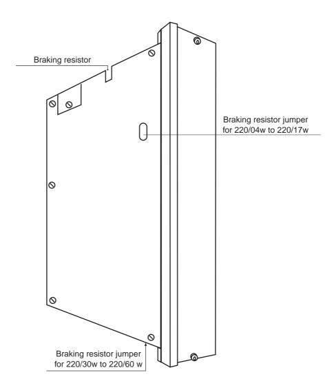
SMT-BM 20 A single-axis rack: Braking resistor jumper closed. BF rack: Braking resistor jumper open.
