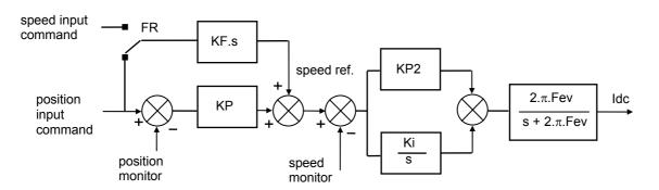
All these gain parameters (KF, KP1, KP2, Ki and Fev) are automatically calculated during the auto-tuning procedure.
