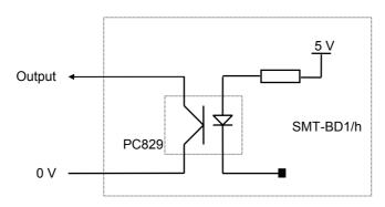
The logic outputs are open collector outputs.
