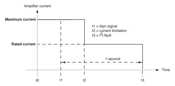
The maximum current duration before the flashing display depends on the value of the **Rated current** and **Maximum current** parameters. This value is calculated as follows:
