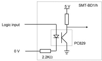
The input voltage corresponding to level 1 is between 5 V and 24 V
