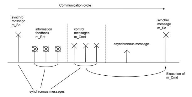
At constant time intervals (cycle time), the NC sends a synchro message m\_Sc and the amplifiers of the same synchronization group acquire their position and send the messages containing their position (m\_Ret). After the reception of the positions, the NC sends the input command messages (m\_Cmd) to the amplifiers of this same synchro group.
